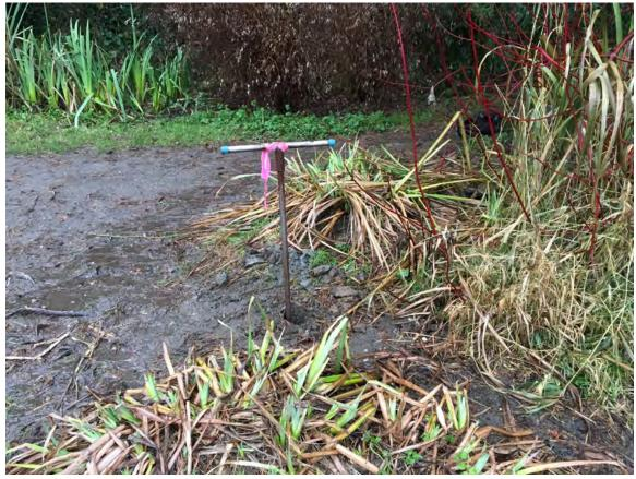
Photo 3 - Test Plot 2. Auger handle is about 5 feet long and is 36 inches in ground where groundwater was encountered.
